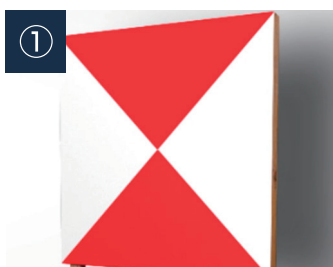
① Placing GCPs on both banks
