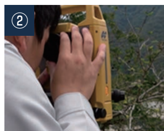
② Surveying the coordinates of GCPs
